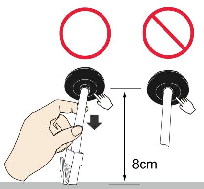
10.Install the silicon seal to the original opening on the bracket.
