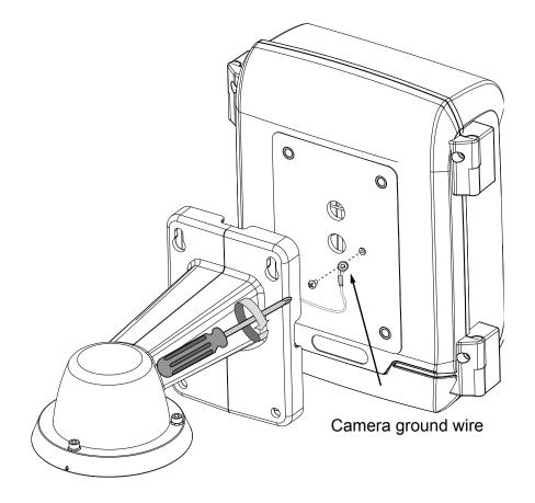
Connect the ground wire to the copper screw hole on the cabinet door.
