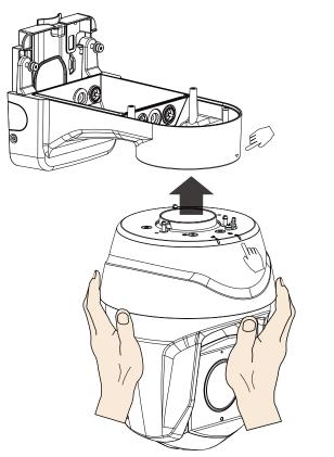
16. Turn the camera clockwise until the second alignment mark on the left aligns with that on the bracket. Secure the connection by fastening 3 screws from the top.
