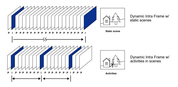
With the H.265 codec in an optimal scenario and when the Dynamic Intra frame and the Smart Stream function are applied, an 80% of bandwidth saving can be achieved compared with using H.264 without enabling these bandwidth-saving features.
