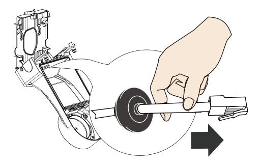
If you purchased the I/O combo cable, the cable will come with the silicon seal.
