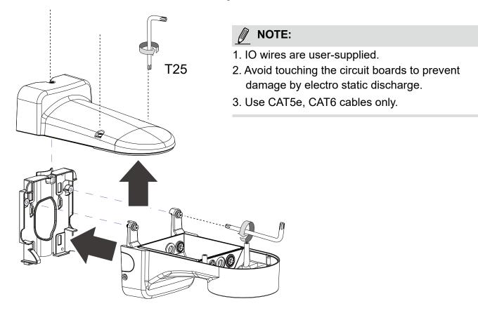
5. Route your I/O combo and Ethernet cables through the drill hole. Secure the bracket to wall using the included screws.
