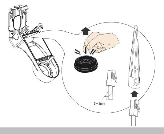
8. Insert and pass the cable through the silicon seal.
