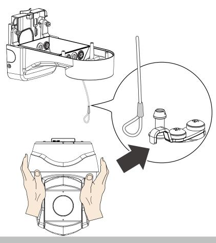
15. Install the camera to the wall bracket by aligning with the alignment mark on the bracket.
