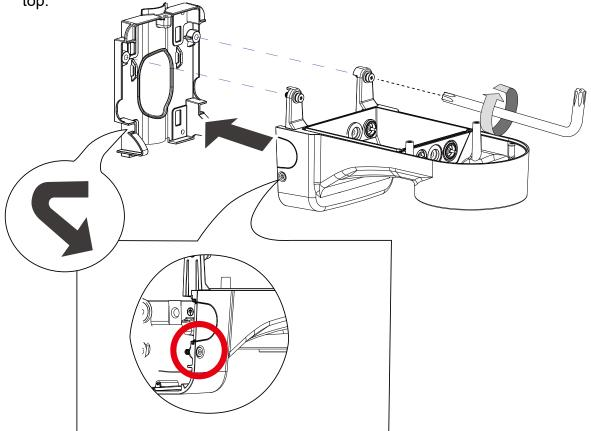
7. Remove the silicon seals from the bracket. Remove the tip of the silicon seal. Insert the RJ45 connector of your Ethernet cable into the penetration cap.
