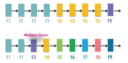
By queuing the old frames from a static scene, both the computing efforts and the size of P frames are reduced. It is beneficial for keeping up with the frame rate requirements.
