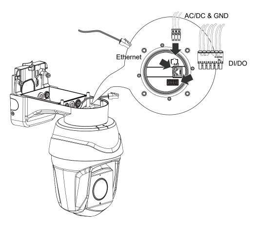
18. Install the top cover of the wall-mount bracket.
